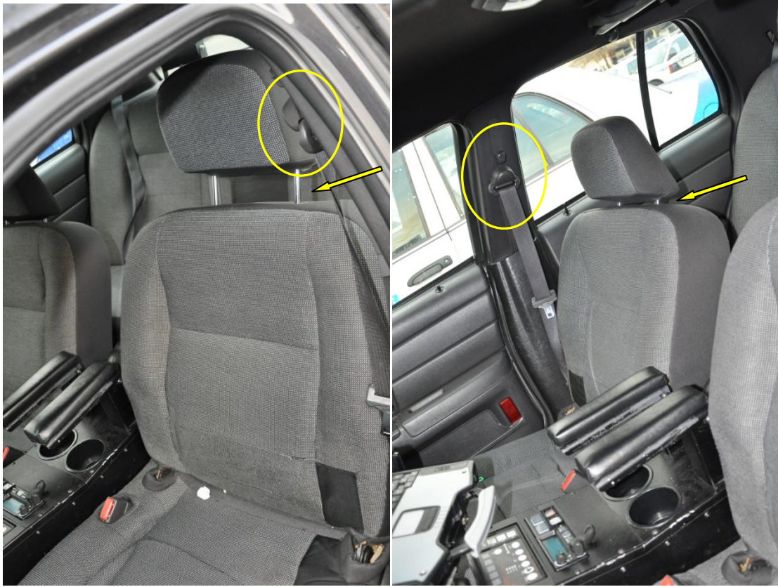
Figure 209: Seat headrest adjustments (arrows) and seat belt height adjustment feature (circled)
