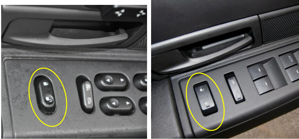
Figure 21: Door locks – Different styles where same action that unlocks the door in one style, locks the door in the other style
