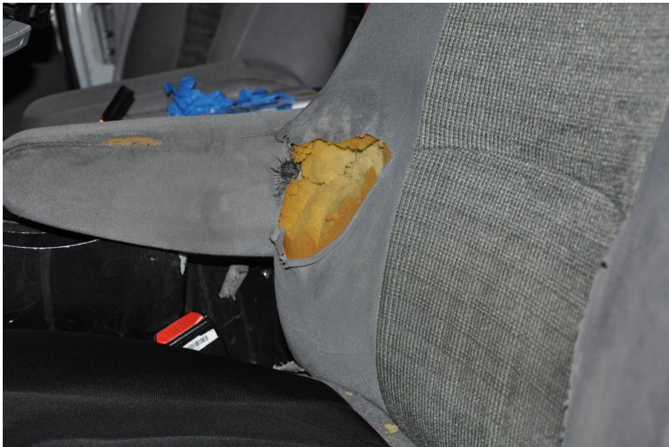
Figure 17: Seat upholstery and foam ripping
