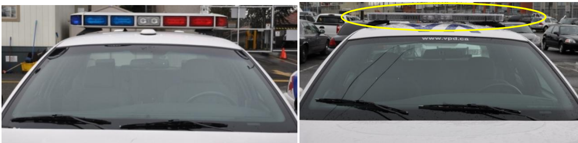
Figure 15: Example of visibility of a police vehicle with a standard light bar (left) in comparison to a low profile light bar (right)
