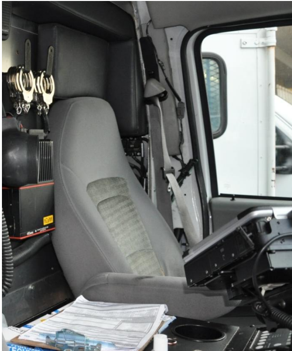
Figure 18: Wagon seat has no backrest adjustability
