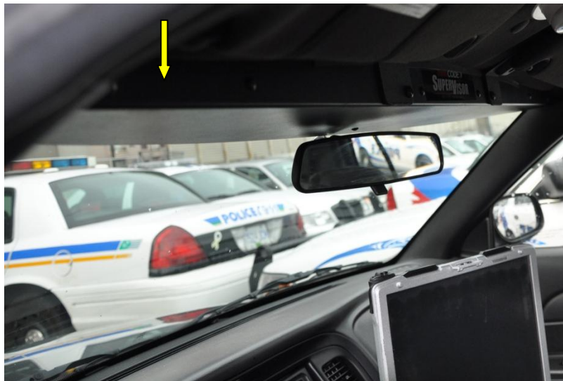
Figure 1 1: Impact of In-car light bar on visibility and relationship to head height
